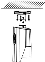
Figure 2-2 Fix the Camera to the Ceiling
